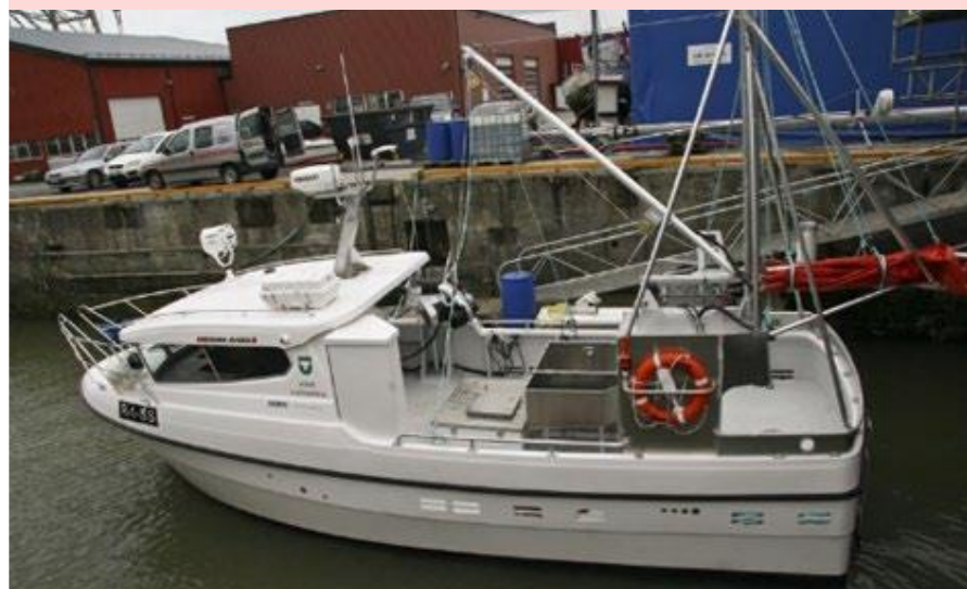
A Norwegian 10.65 speed sjark vessel, operating in the North Sea, providing validation of the hull coating and low-cost sensors technologies
