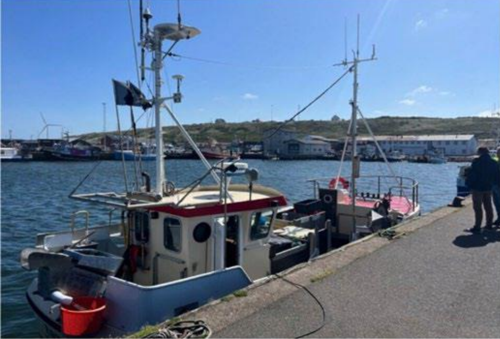
A Danish-registered hybrid methanol / electric powered 10m line-fishing boat, with electric hydraulics and hydrofoils, operating in the North Sea (Technology 1).
